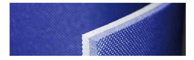
LDPE foams are semi-rigid. In order to impart more softness and resiliency to LDPE foams polar copolymers in the range between 10 % - 50 % are often added as part of the formulation. Suitable polar copolymers are poly butyl acrylat, poly methyl acrylat, poly ethyl acrylat and poly vinyl acetat. In order to be fit for use in their specific applications and markets, such as automotive, building and aerospace, excellent low temperature properties are often very important.
