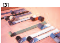
Illustrations: [1], [2] low-temperature fracture of a sample; [3] unrolled lengths of various sheets at low temperature
